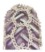
H-Pattern Studded Grader Chains are made with easy to replace, double studded twist link cross chains. The H-Pattern provides less side slip, more traction and better tire protection than studded ladder style. Made with fully case hardened strong boron steel.
