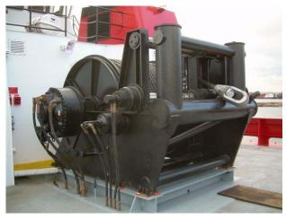
JonRie InterTech introduces its NEW Series 525 Hydraulic Towing Winch. The Winch boasts a line pull of 150,000lbs. and a line speed of 30 FPM. The winch also features an independent drive level wind so the speed can be adjusted to hold the cable to the flange for an even spool. Also featured is an integral H-Bitt to reduce the countering loads on the level wind and can also be used for towing. The Series 525 is designed to handle 2 1/2" wire.
