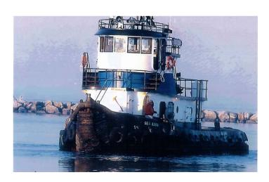
JonRie InterTech installed its Series 500 Towing System on the tug Sea Lion. The Winch boosts a line pull of 60,000lbs. And a line speed of 30 FPM. JonRie also provided a series 200 Hydraulic Power Unit and Controls.
