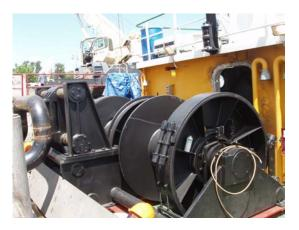
JonRie InterTech installed its new Series "500" Double Drum **Hydraulic Towing Winch on the** ASD Don Alfredo for Harbor Fuel Services of San Juan. The Winch boasts a line pull of 75,000lbs. and a line speed of 30 FPM. JonRie also provided a series 300 75HP Hydraulic Power Unit and a JonRie Series 900 Control system.
