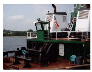
JonRie InterTech installed its Series 500 Towing System on the new tug Donald C. The Winch boosts a line pull of 100,000lbs. And a line speed of 30 FPM. Jon-Rie also provided a series 200 Hydraulic Power Unit and Controls.
