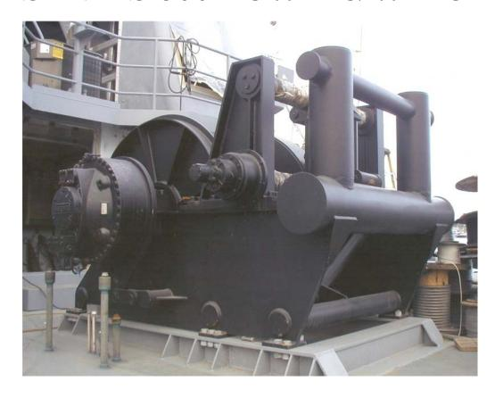
JonRie InterTech also introduces its NEW Series 500 Hydraulic Towing Winch. The Winch boasts a line pull of 100,000lbs. and a line speed of 60 FPM. The winch also features an independent drive level wind so the speed can be adjusted to hold the cable to the flange for an even spool. Also featured is an integral H-Bitt to reduce the countering loads on the level wind and can also be used for towing.
