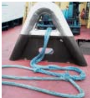
Strop to main line connection.
