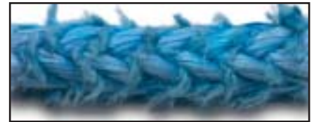
FIG. 3 Severely abraded rope
