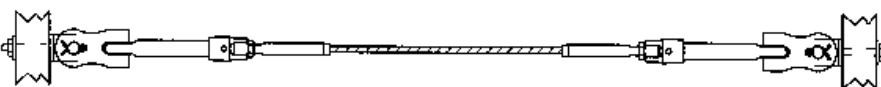
5. Sealoc toggle/swage turnbuckle each end for extra tension on longer runs with anchor bolt connections.
