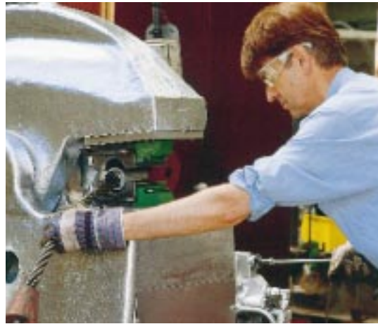
500 tonne press for swaging fittings on wire rope
