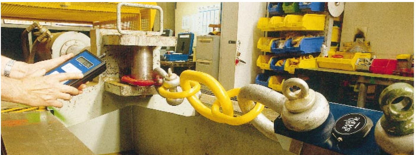
Proof Load Test using Bridon telemetry load indicator.
