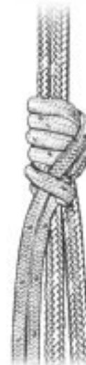
A "kreutzklem" is a popular substitute for the Prusik hitch in the secured static footlock system.
