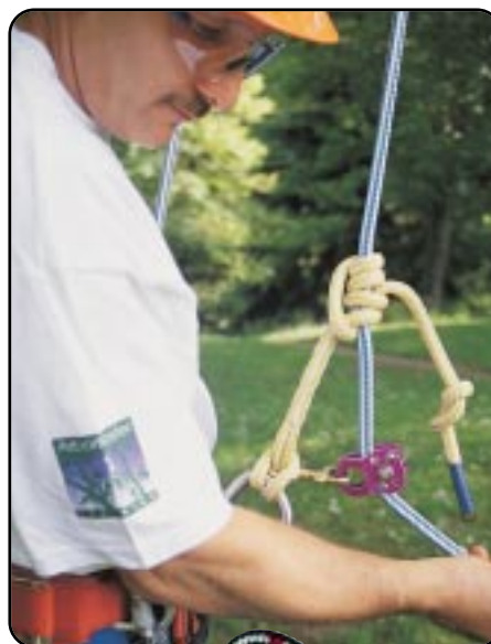
ArborMaster's various color combinations work well together when used in the split-tail climbing system.
