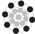
ArborMaster® premium 16-strand braided polyester construction. With a uniquely stabilized nylon core.
