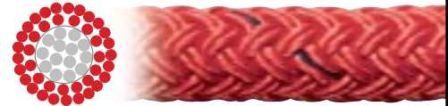
STABLE BRAID™ 2-in-1° double braid construction consisting of a braided polyester cover over a braided polyester core.
